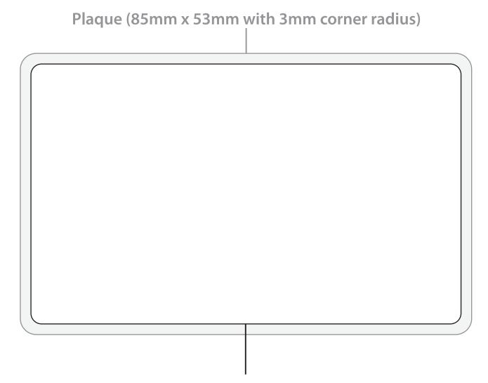
Inner Design Size =  $81 \text{mm} \times 49 \text{mm}$ , corner radius 2 mm.
